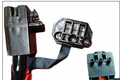
Photo 2 Pump connector with transport cover
