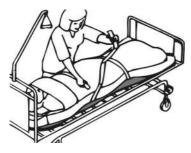
Secure the user to be evacuated with both straps.
