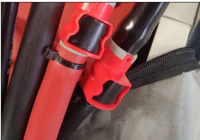
Photo 3 Hose set connectors The hoses have three quick release connectors that should be checked in the event of an alarm for a drop in air pressure. Check that the O-rings of the connectors are not missing, incorrectly fitted or damaged.
