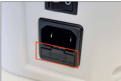
Figure 1 The pump fuse is inside a cover, located under the power connector. The cover can be twisted open with a small screwdriver or similar.
